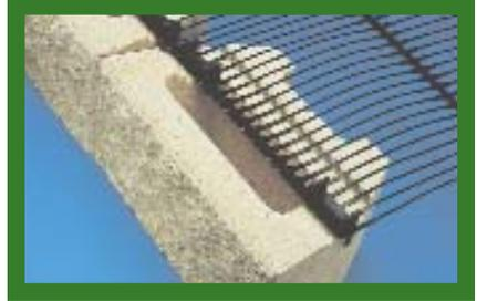
Prior to placement of additional courses, two Connectors are inserted into each preceding Mesa Unit. The flags or exposed portion of the connector will create the alignment with the unit above. If the design dictates the need for a geogrid at a particular elevation, the Tensar Geogrid will be installed with the Mesa Connectors penetrating through the geogrid apertures. Snug the geogrid against the connector teeth, and then drive the connector the rest of the way using a rubber mallet.
